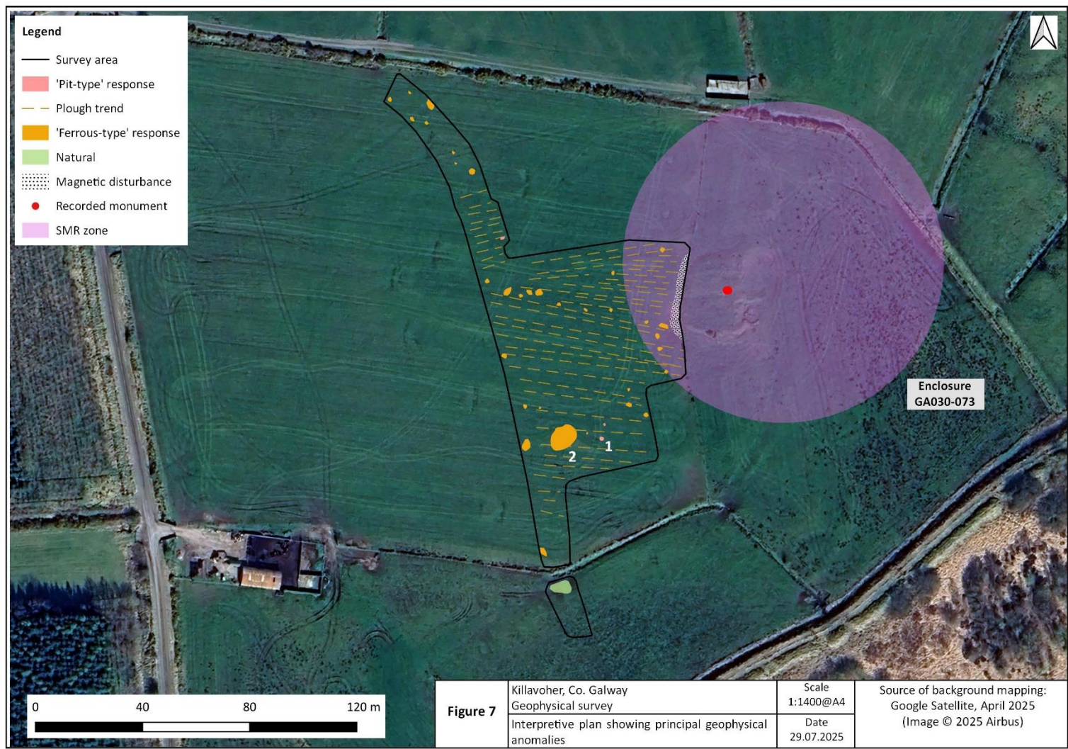
Figure 7. Interpretive plan showing principal geophysical anomalies.
